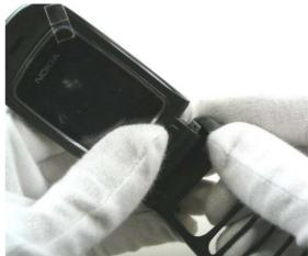
Caution: Do not separate the two assemblies after the hinge is opened.
