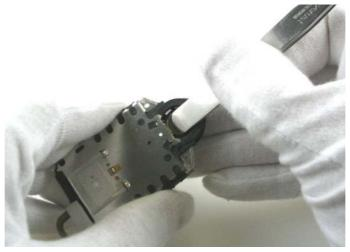
Note for Assembly: Do not to damage the earpiece spring contacts once it has been removed.
