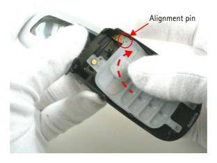
Note for Assembly: Be careful of alignment pin that retains the keymat in C-cover.
