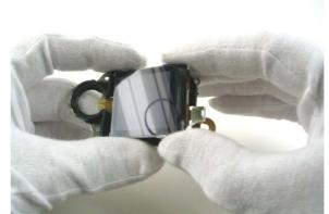
Caution: Do not damage the LCD flex cable while separating the components.
