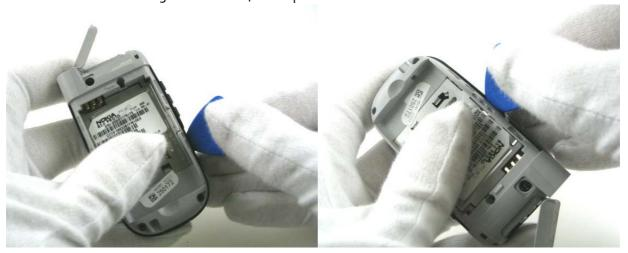
b. Remove the D-cover by lifting upward and then sliding off of the B/C-cover assembly, as shown below.
