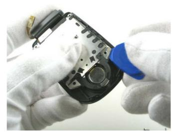
c. Using the SRT-6 tool unsnap LCD connector and separate the LCD display assembly from the display shield assembly.
