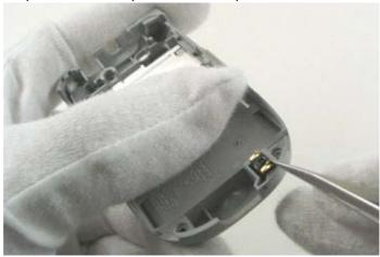
Note for Assembly: Once removed, always replace the microphone module with a new assembly.
